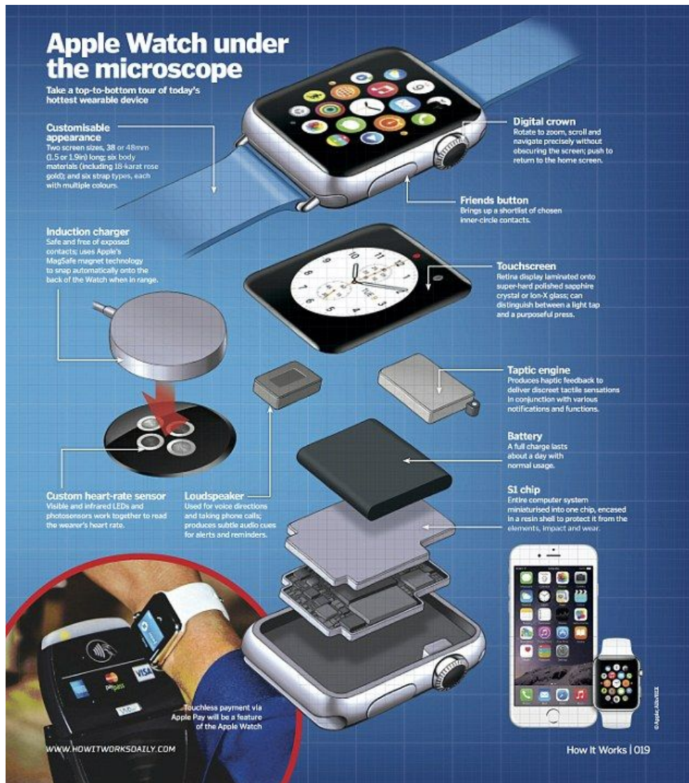
Figure 2. Interior components of Apple Watch. Reprinted from “Take a peek inside the Apple Watch” by V. Wollaston, 2015.
